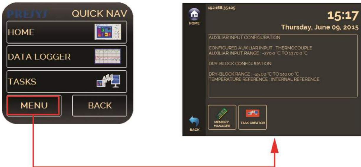
Fig. 07 - Quick Navigator and Secondary Menu
