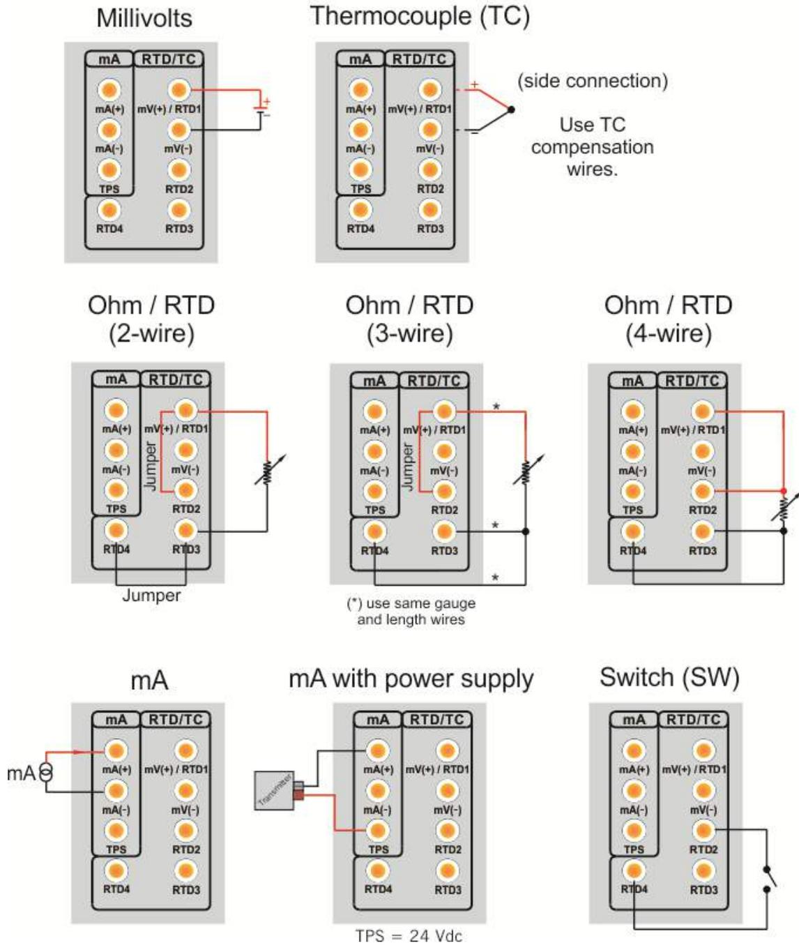
Fig. 15 - Input Connections
