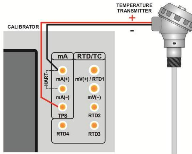
**Fig. 19 - Transmitter Powered by the Calibrator Itself (TPS)
