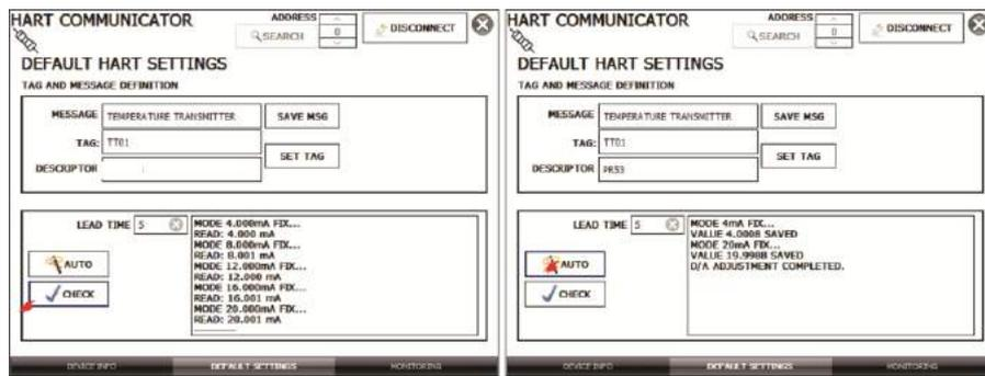
Fig. 24 - Checking / Adjusting the mA HART® Transmitter Output
