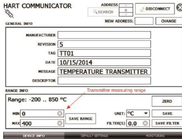
Fig. 21 - Adjusting the measuring range of the HART® transmitter
