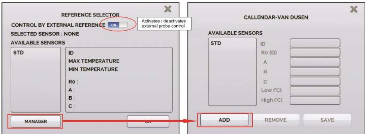
**Fig. 09** - Adding a new Reference Sensor
