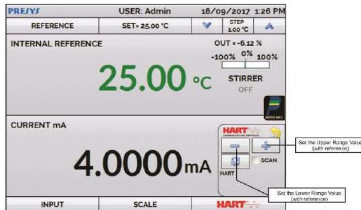
Fig 22 - Quick HART® Adjustment with Reference
