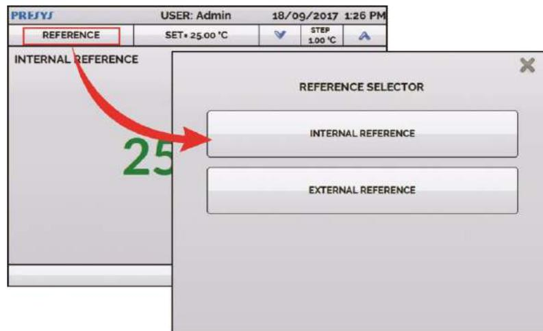
**Fig. 08** - Choosing the Type of Temperature Reference
