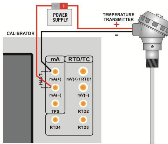
**Fig. 20 - Transmitter Powered by an External Power Supply
